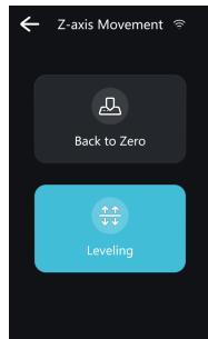
1. After unscrewing the leveling screws, press "Leveling" to keep the platform and the print screen parallel.
