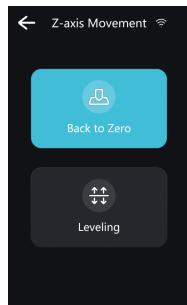
3. Press "Auto-homing", move up the z-axis to a proper position, and then tighten the fixing screws at both ends of the resin vat.
