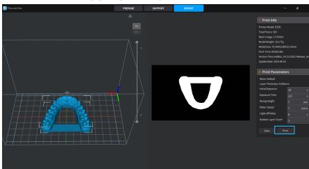
4. Waiting for the auto slicing to complete (you can adjust the print parameters as required).
