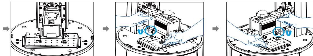
2. Gently press the platform and tighten the 4 screws clockwise and diagonally, and the platform will be successfully leveled.
