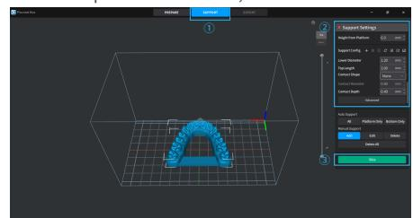
3. Add bracket to the model (skip steps ① and ② if no bracket is added).
